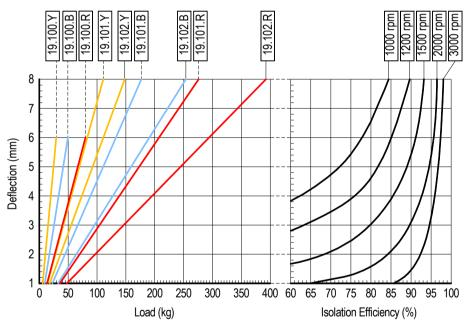
Isolation efficiency is based on dynamic rather than static stiffness for accurate calculation of system performance.
