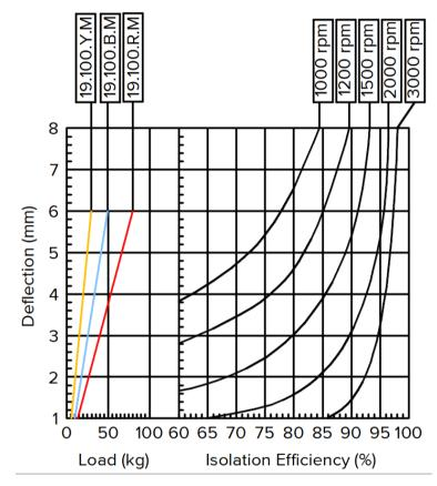
Isolation efficiency is based on dynamic rather than static stiffness for accurate calculation of system performance.
