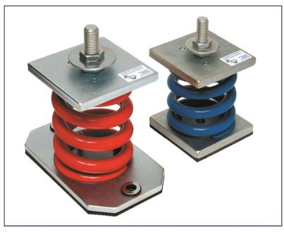
Originally designed for use with Type IPF Inertia Pouring Frames, the OS Mountings are now widely used to isolate vibration from every conceivable type of rotating and reciprocating machine. Where control of transient motion is required Open Spring Mountings can be used in conjunction with our Viscous Dampers Type SFD.
