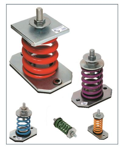
This unique range of Open Spring mountings uses integral rubber end fixing of the springs which sets them apart from all other designs. Larger capacity open spring mountings use rubber grommets and base pads to ensure no direct metal path between the machine and the seating, thus enhancing high frequency noise isolation.
