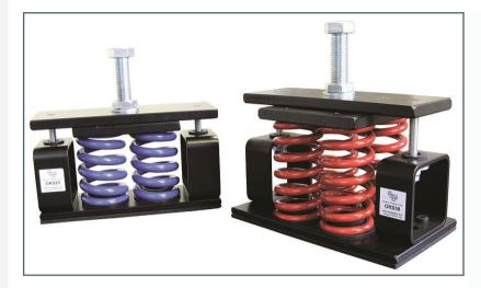
The ORS mounting has been designed specifically for applications where transmission of low frequency machinery vibration to a building structure must be reduced to avoid physical damage or annoyance to the occupants.
