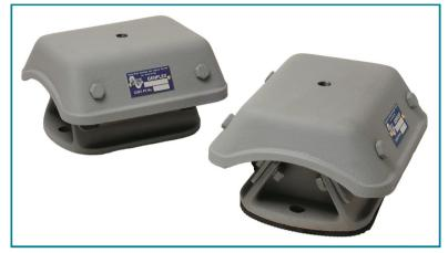
Genflex mountings employ the well proven inclined rubber element design to achieve much higher deflections compared to simple rubber in compression devices and therefore providing superior isolation of low frequency vibration.
