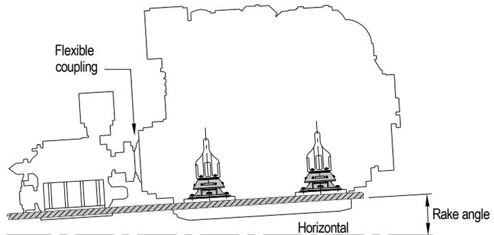
**Marine diesel propulsion engine on T3 isolators**
