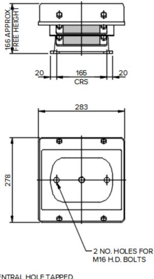
CENTRAL HOLE TAPPED FOR M20 FIXING BOLT
