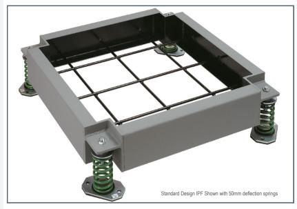
Inertia Pouring Frames have been developed for use with machines which produce high levels of vibration or those which are subjected to external forces or are simply unstable when mounted directly on spring or rubber mountings.
