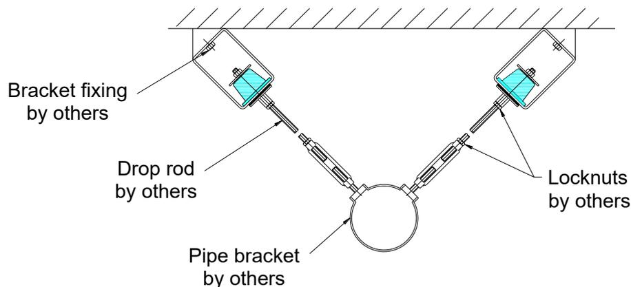
Adjustment on rubber hangers should be done by adjusting the stud length through the turnbuckle to change the length of the drop rod. Once this adjustment has been achieved the second locknut should be secured against the turnbuckle.
