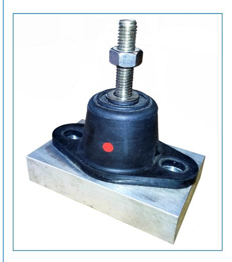
Marine Rubber Turret mountings are designed to provide superior attenuation of medium to high frequency vibration and noise emanating from a wide range of motor driven machines particularly axial and centrifugal fans.
