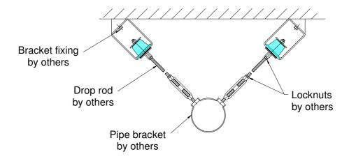
Adjustment on rubber hangers should be done by adjusting the stud length through the turnbuckle to change the length of the drop rod. Once this adjustment has been achieved the second locknut should be secured against the turnbuckle.
