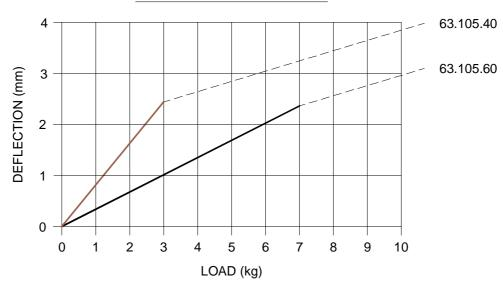
Small Rubber Mountings should not be used in tension or exposed to contamination by mineral oils. For full installation instructions please refer to our data sheet DS010.
