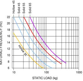
The maximum loads stated above are calculated at 8 mm vertical deflection and are subject to a production tolerance of + / - 20%. Studflex pads should be protected from severe contamination by mineral oils.
