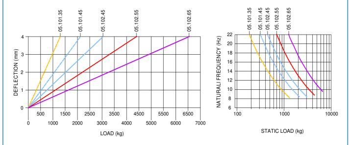
The maximum loads stated above are calculated at 4 mm vertical deflection and are subject to a production tolerance of + / - 20%. Studflex mats should be protected from severe contamination by mineral oils.
