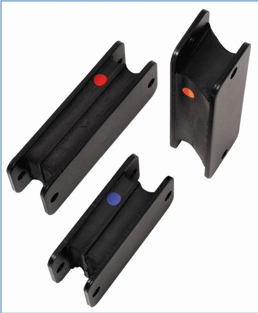
Rectangular mountings, also known as sandwich mountings, are widely used for mounting engines in road vehicles and mobile construction plant. In the larger sizes they are used as vehicle suspension springs and as mountings for acoustic chambers, hoppers and various types of heavy plant installation.
