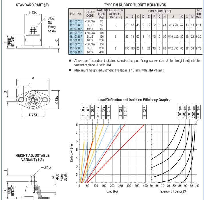
Isolation efficiency is based on dynamic rather than static stiffness for accurate calculation of system performance.
