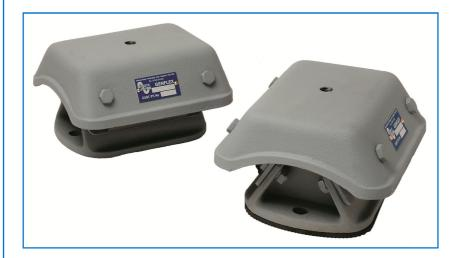
Genflex mountings employ the well proven inclined rubber element design to achieve much higher deflections compared to simple rubber in compression devices and therefore providing superior isolation of low frequency vibration.
